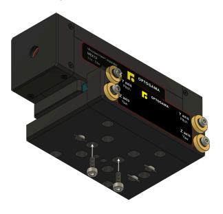
2. When the expander is properly fixed, place the manual stage (with fixed expander) on the bottom side and fix it with Metric M6x1.0 or Imperial 1/4"-20 screws. It can be fixed on both Metric and Imperial optical breadboards and tables:
